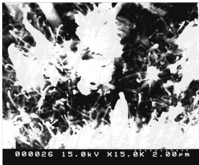
Figure 1. SEM images of the CVD-grown BN nanotubes from B_4N_3O_2H precursor.
